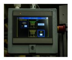
The number of rows, number of layers and pack pattern can be stored and recalled as necessary
