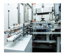
The in-feed conveyor attached to the machine can be integrated with the discharge conveyor of the blow moulding machine from any direction
