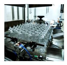
Layers are formed as per the selected pack pattern. The complete layer is automatically ejected in the event of a fallen or missing bottle.
